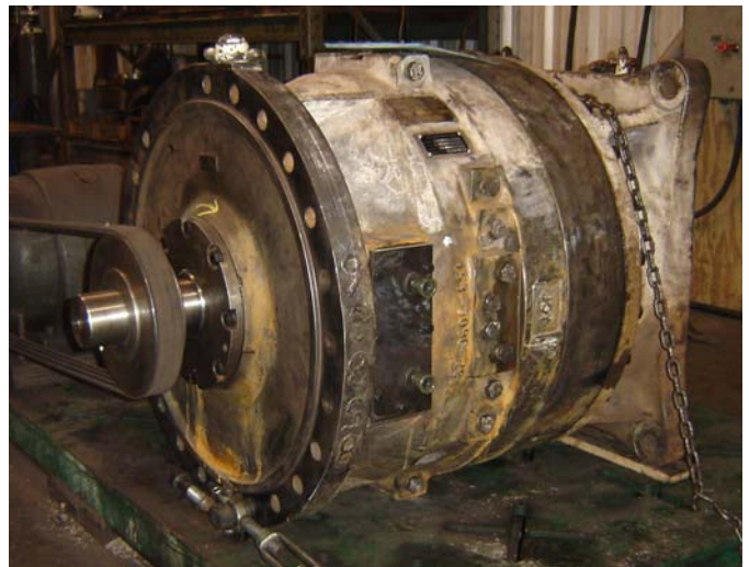
Figure 2. Gearbox On Test Stand For No Load Spin Test.
