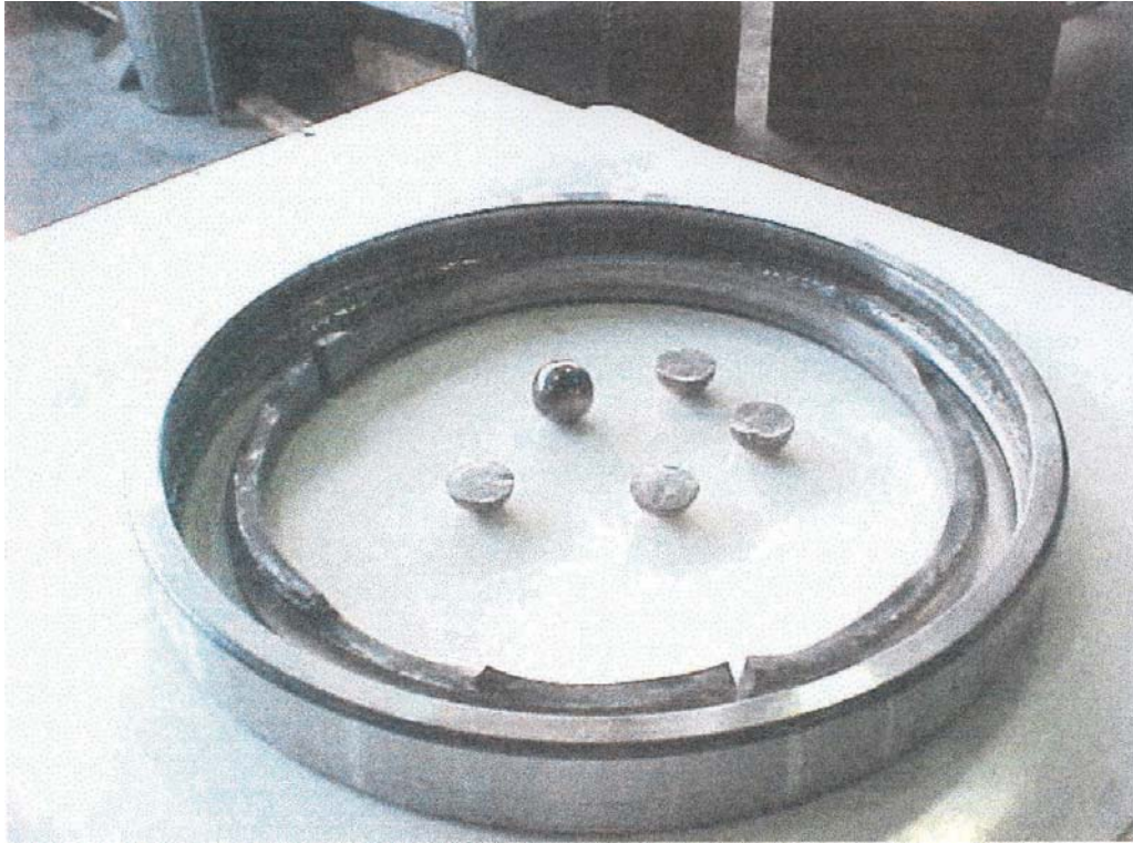
Figure 18. Bearing Removed from Service Referenced in Figure 16. Outer Race Spalling Over Full 360 Degree Arc. Outer and Inner Races Cracked. Two (2) Balls Cracked
