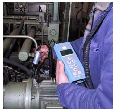
Figure 5 - dB \mu V levels on hydraulic pump motor
