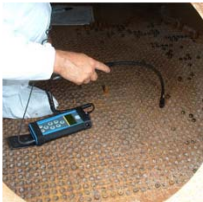
Figure 13 - Inspecting heat exchanger tube sheet and end plate for leaks
