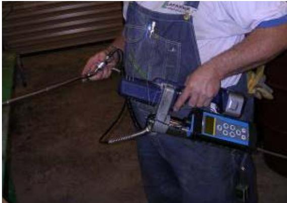
**Figure 8 - Ultrasonic lubrication at Lafarge North America**
