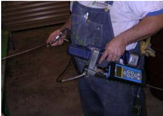
Figure 8 - Ultrasonic lubrication at Lafarge North America
