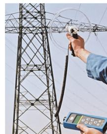
Radio and TV interference are common complaints from local cable companies. Often the source can be traced to a faulty transformer or a failed lightning arrestor. Pinpointing the culprit is quick
